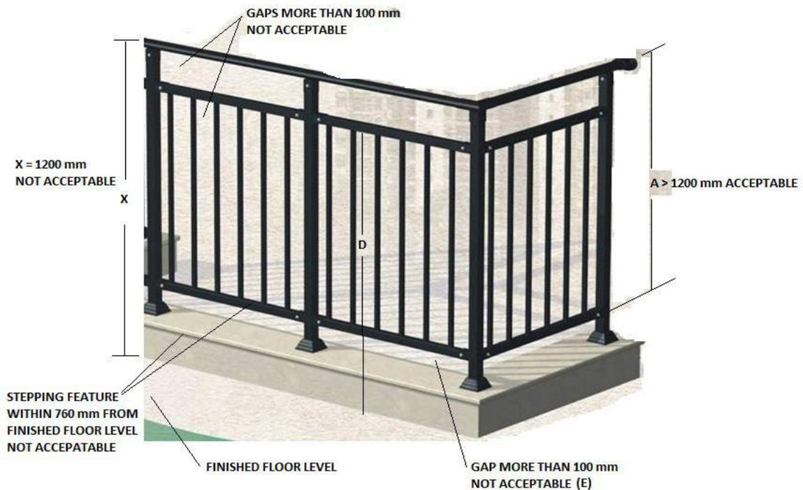
**Figure 1.16.b.: Balcony Railing Specifications**
